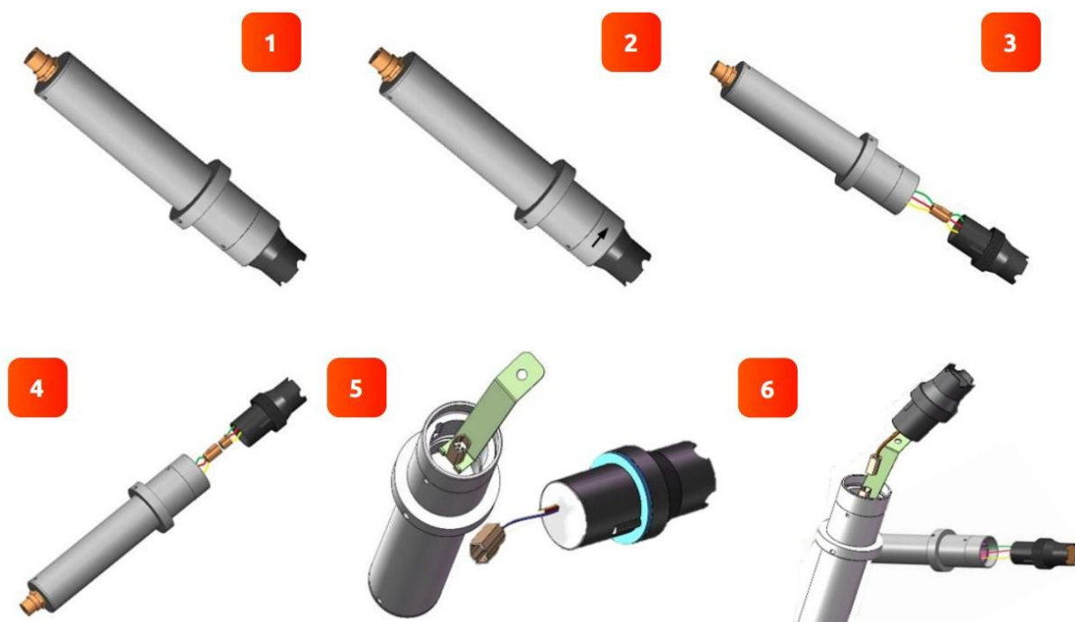
Figure. 82 - Replacing EH-765-01 pH and Oxidizer Electrode Head
