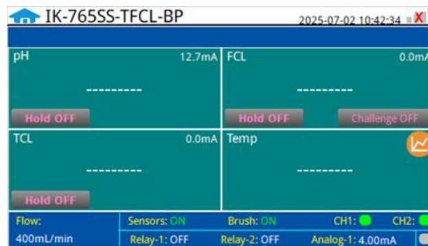
Figure. 25 - Numeric Display "---" with Flow
