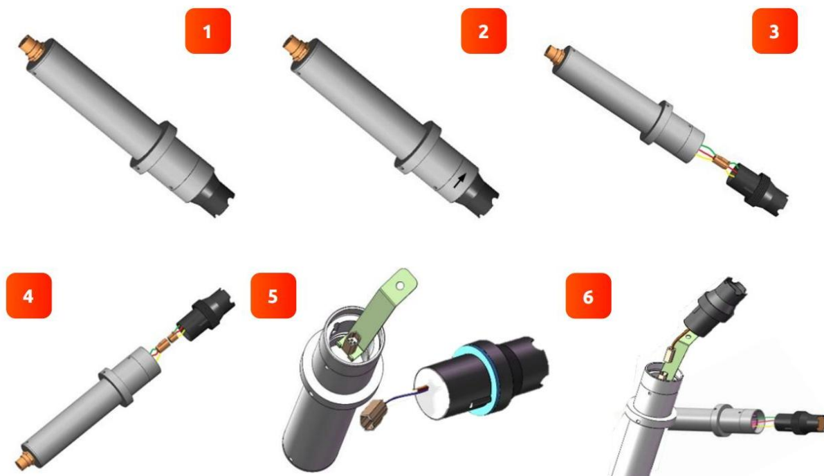
Figure. 80 - Replacing EH-765 pH and Oxidizer Electrode Head
