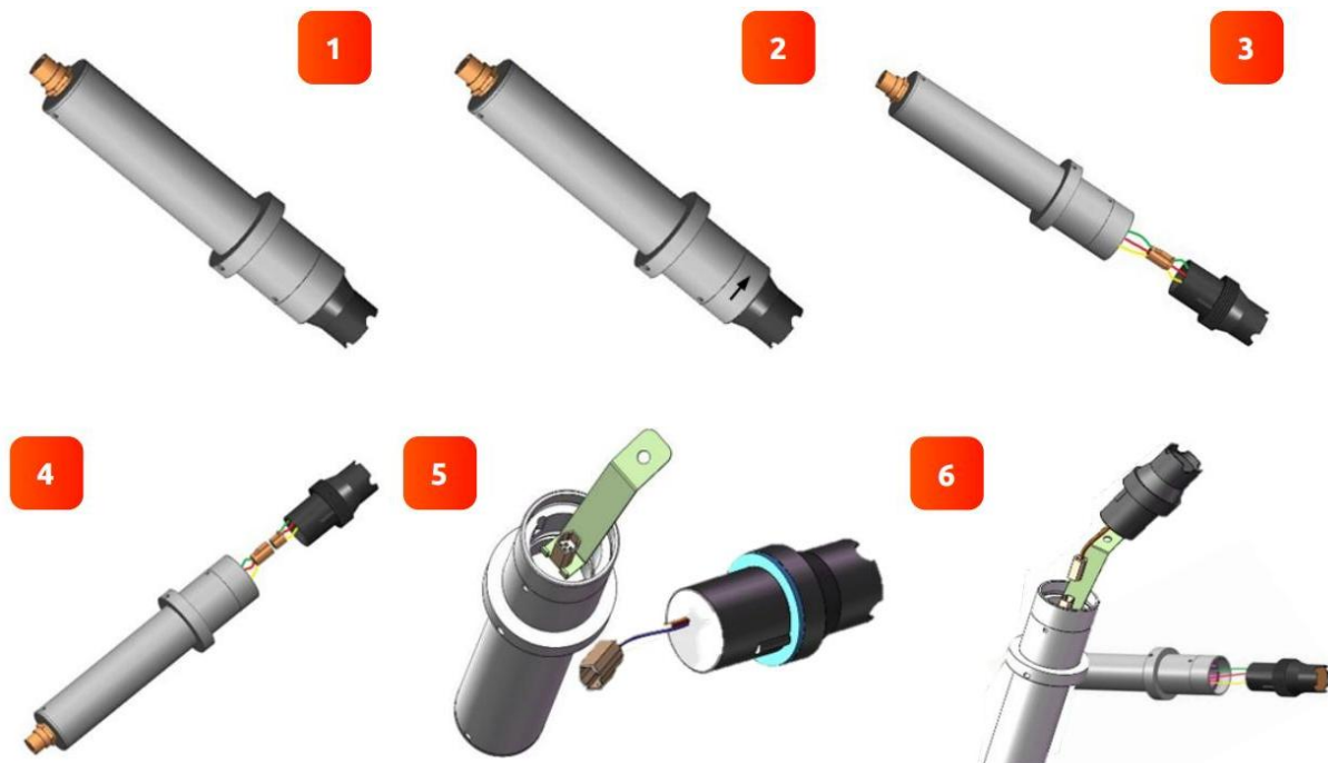
Figure. 86 - Replacing EH-765 pH and Oxidizer Electrode Head
