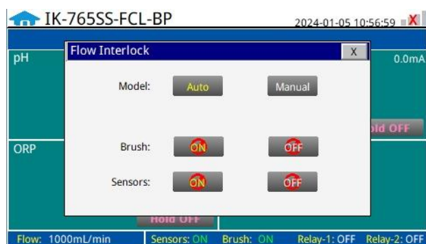
Figure. 29A - Flow Interlock Control - Automatic Mode
