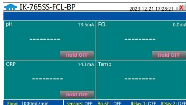
Figure. 28B - Numeric Display "---" Flow &lt;50mL/min
