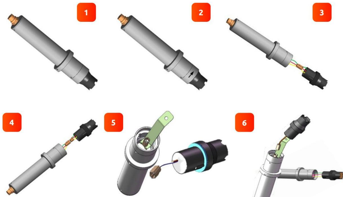
Figure. 79 - Replacing EH-765 pH and Oxidizer Electrode Head
