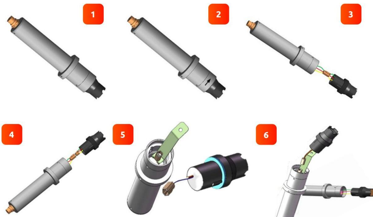
Figure 55 - Replacing EH-765-O3 pH and Ozone Electrode Head
