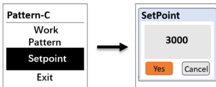
Figure. 2C - Flow Control (C) Operating Mode with User Defined Setpoint
