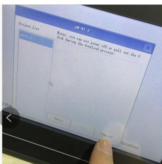
6. During the HMI restarting process, you can pull out the U disk. If it is not pulled out, when the update screen appears again after restarting, please click "NO" to pull out the U disk.
