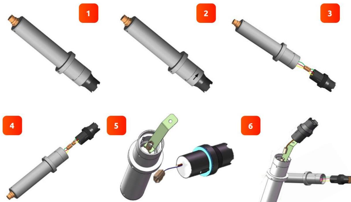
Figure. 52- Replacing EH-765 pH and Oxidizer Electrode Head
