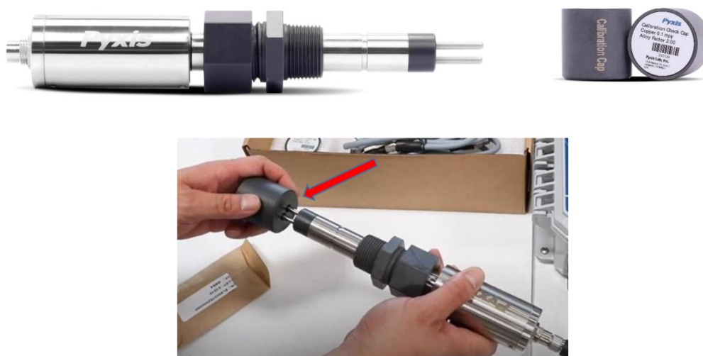
Figure. 34 Installing the Calibration Check-Caps onto CR-300 with Electrodes
