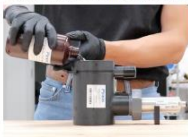
Add Calibration Standard (500mL)
