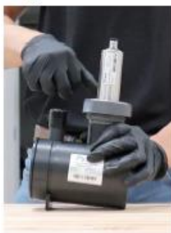
Tighten Sensor Nut
