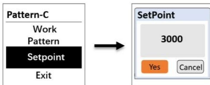
Figure. 6 - Flow Control (C) Operating Mode with User Defined Setpoint
