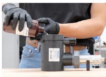
Add Calibration Standard (500mL)
