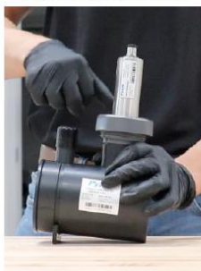
Tighten Sensor Nut
