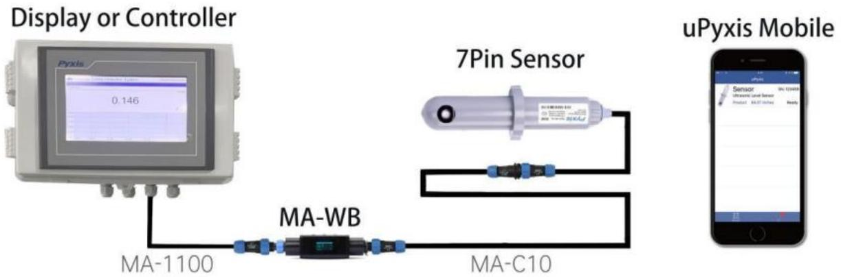
**Connection Diagram #2 (Using USB Connection for Power Supply)**
