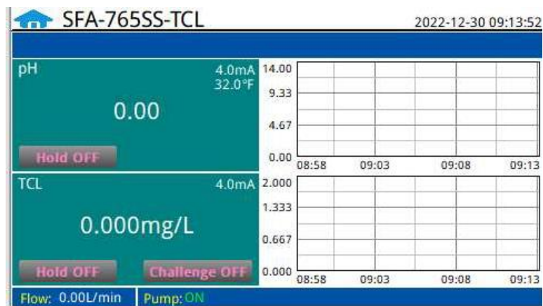
Figure. 12 - Chlorine Challenge OFF Status
