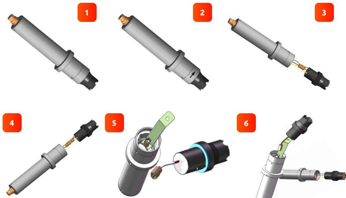
Figure. 43 - Replacing EH-765 pH and Oxidizer Electrode Head
