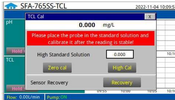
Figure. 27 - Total Chlorine Calibration of ST-765SS-TCL
