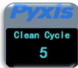
Figure 8. – Programming the Clean Cycle Frequency
