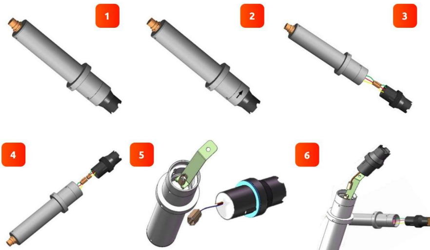
Figure. 89 - Replacing EH-765 pH and Oxidizer Electrode Head
