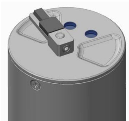
Figure 29 Set wiper arm to horizontal position
