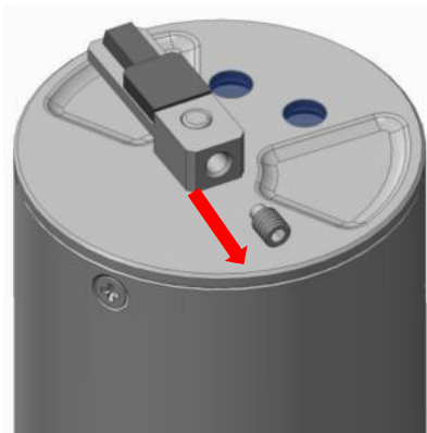
Figure 30 Remove the M2 screw
