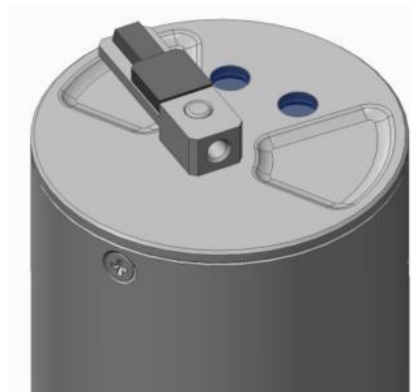
Figure 32 Install the new wiper arm
