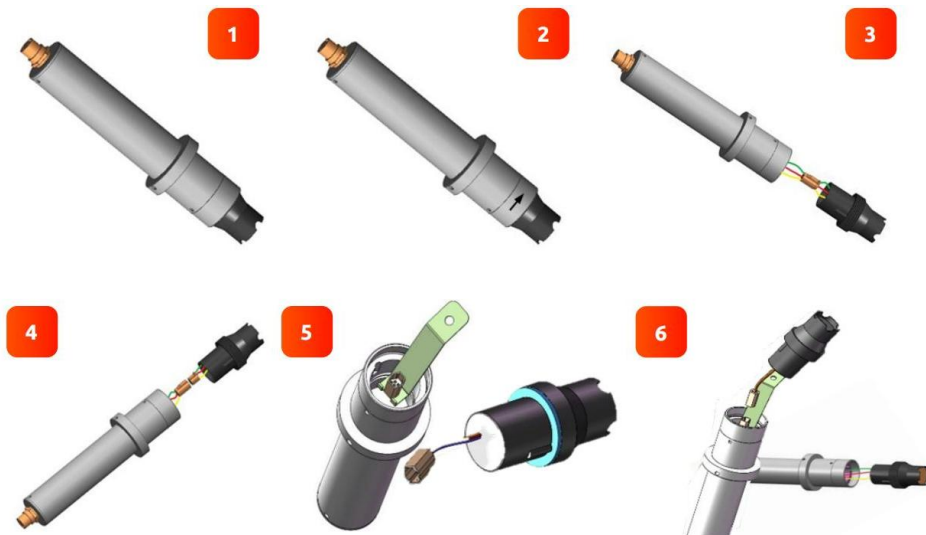
Figure. 75 - Replacing EH-765-01 pH and Oxidizer Electrode Head
