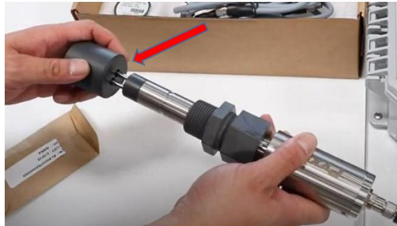
Figure. 24 Installing the Calibration Check-Caps onto CR-300 with Electrodes
