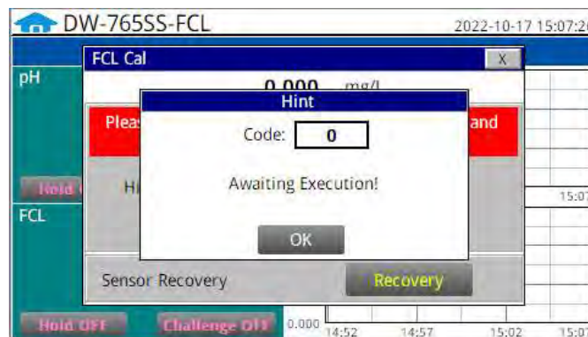
Figure. 25 - Awaiting Execution Screen of FCL Calibration
