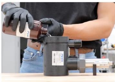
Add Calibration Standard (500mL)
