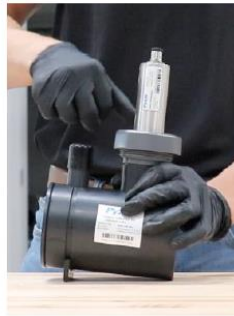
Tighten Sensor Nut
