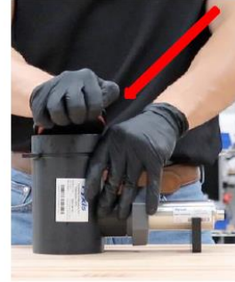
Position Vertically and Remove Lid
