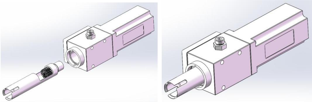
**Step 6.** Reinstall the sensor to the position as shown in the picture.
