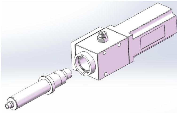
**Step 3.** Insert the extraction tool with the slotted end first until the head of the tool snaps onto the collar of the brush.
