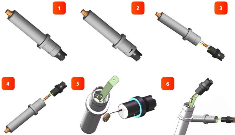
Figure. 75 - Replacing EH-765-01 pH and Oxidizer Electrode Head
