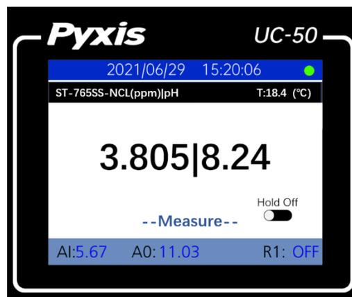
UC-50 controller supports manual selection of the probe type or automatic identification of the probe type. Please use the up/downs keys to select the correct probe type or select Auto Discover.
