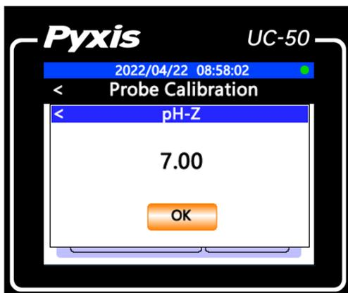
Select the OK button on the **probe Calibration** confirmation page. The UC-50 controller sends the pH-Z calibration command to the ST-765SS probe and waits for the probe calibration result. The probe calibration result will be automatically displayed on the calibration interface.
