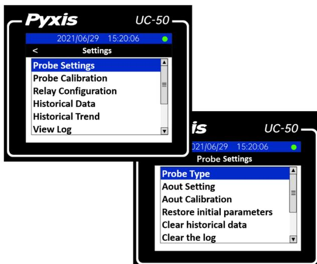
The UC-50 is preset to be connected to the ST-765SS-NCL probe when it leaves the factory. After the UC-50 is turned on, the main interface of the UC-50 will display the Monochloramine concentration, pH value and temperature of the tested solution. The green dot in the upper right corner of the UC-50 main interface indicates that the UC-50 is operating normally. If used, the 4-20mA input signal, 4-20mA output signal and relay output states are displayed at the bottom of the UC-50 main interface.
