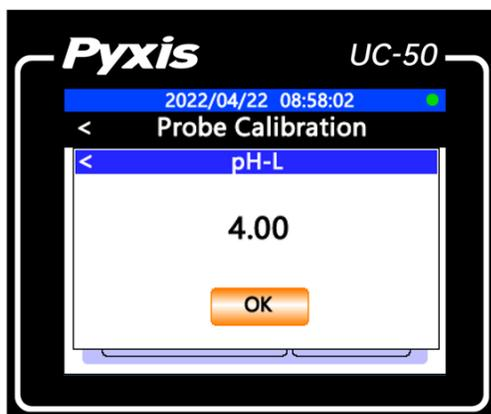
Select the OK button on the **probe Calibration** confirmation page. The UC-50 controller sends the pH-L calibration command to the ST-765SS probe and waits for the probe calibration result. The probe calibration result will be automatically displayed on the calibration interface.
