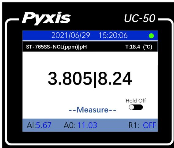
Long press **OK** button for 3 seconds on the main interface to open the **HOLD - ON/OFF** page. The cursor shows **black** is the selection mode, and **blue** is the editing mode. Click the **OK** key to enter the editing mode, and the **up/down** keys can be used to adjust the value of the setting item. Once set where desired, click the **OK** button to start the **HOLD-ON** function.
