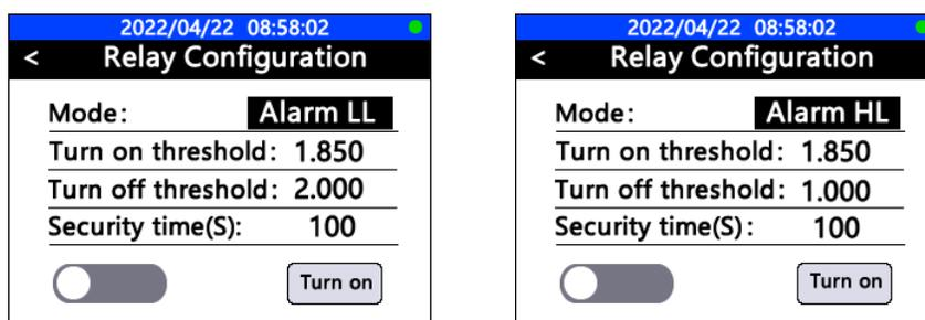
**\*NOTE\*** - If the user program security time has been reached but the alarm Lower limit or alarm higher limit have not been met, the UC-50 main screen measurement values will turn **RED**.
