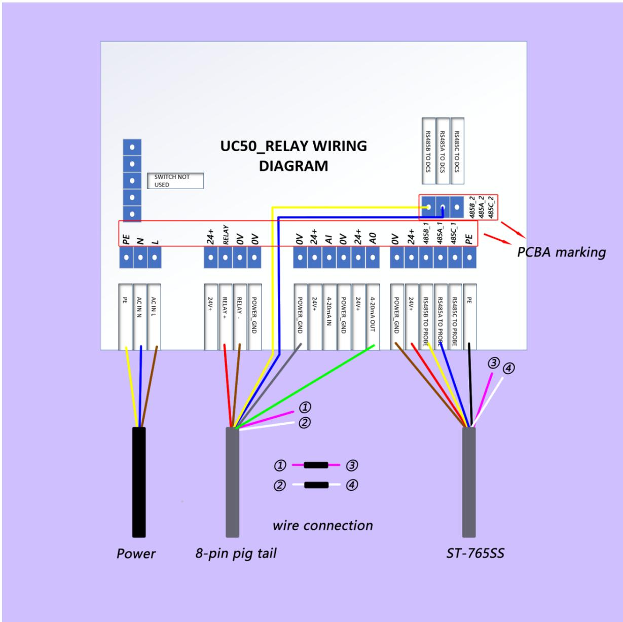
**UC-50 OUTPUT SIGNAL/RELAY WIRING DETAILS AND 4-20mA RANGES.**
