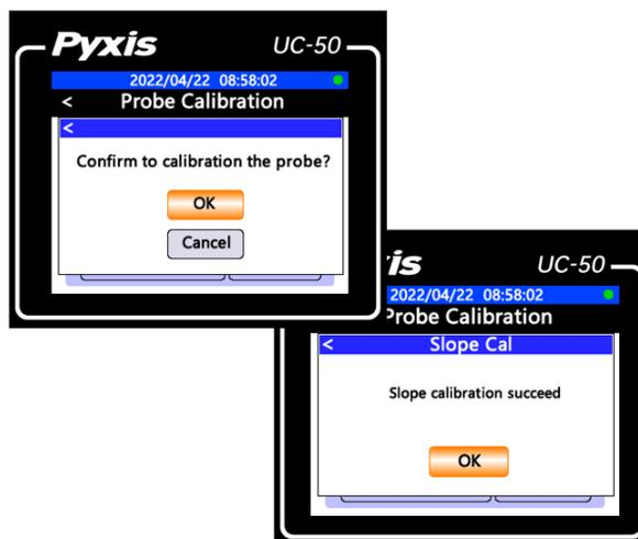
**\*NOTE\*** The ST-765SS-NCL must be slope calibrated in the FR-50 flow reservoir provided with the sensor and have consistent flow.
