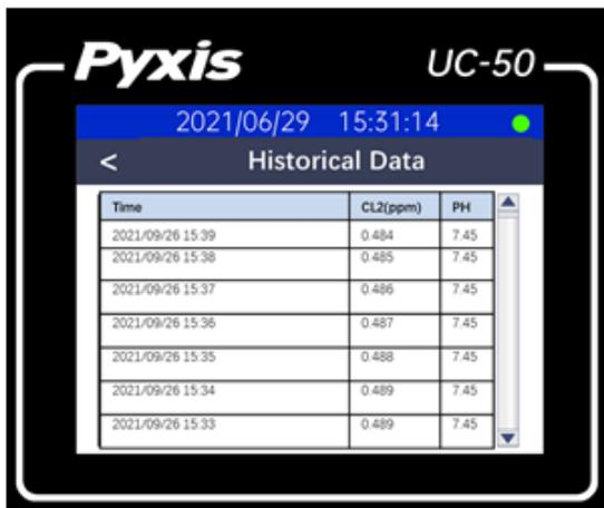
Select the **Historical Trend** on the setting interface of the UC-50 controller. You can view the historical measurement data saved by the UC-50 controller in the form of a trend graph. Use the up and down keys and the confirm key to select to view the data of the last day, week or month.
