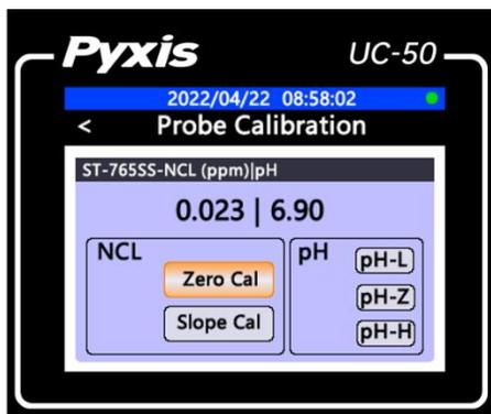
Select the OK button on the probe calibration confirmation page. The UC-50 controller sends the **Zero calibration** command to the ST-765SS probe and waits for the probe calibration result. The probe calibration result will be automatically displayed on the calibration interface.
