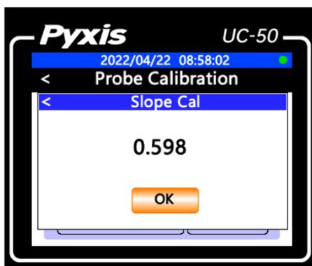
Select the OK button on the probe calibration confirmation page. The UC-50 controller sends the **Slope calibration** command to the ST-765SS probe and waits for the probe calibration result. The probe calibration result will be automatically displayed on the calibration interface.
