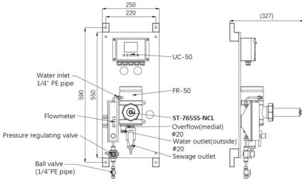
**IK-765SS Series UC-50 Display/Data Logger Dimensions (mm)**
