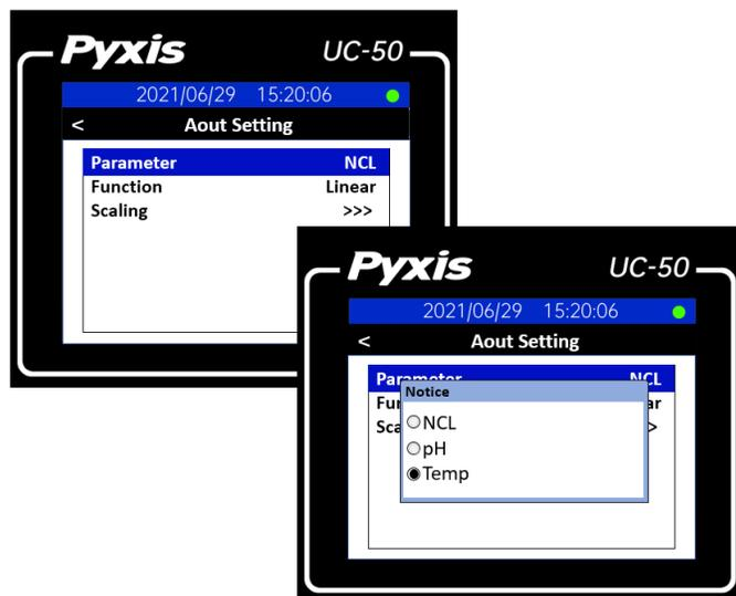
Click **Scaling** option to enter the 4-20mA span interface. You can change the Monochloramine, pH or Temperature value corresponding to the 20mA output to the same or lower default value as seen in the figure below. Click the **OK** button when complete.
