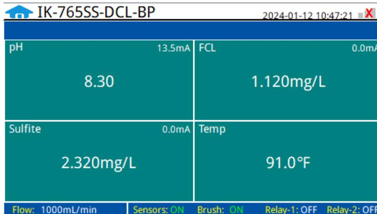
Figure. 12 - Real-time monitoring screen
