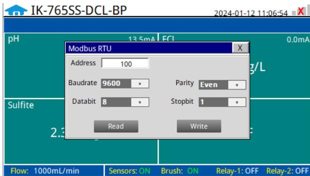
Figure. 37 - Modbus RTU
