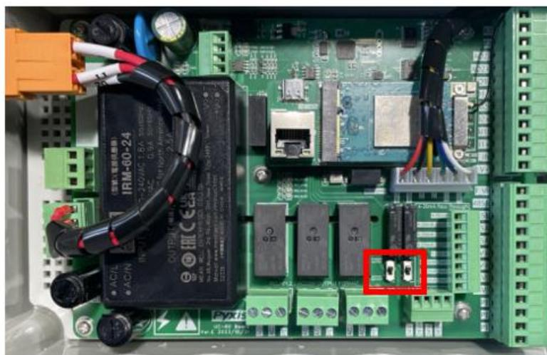
Figure. 19 – Relay Active/Passive Toggle Switch on UC-80 Terminal Board
