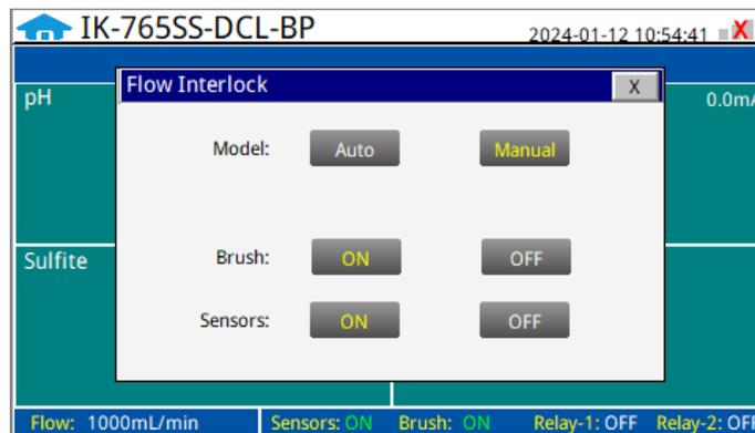
Figure. 17 - Flow Interlock Control - Manual Mode
