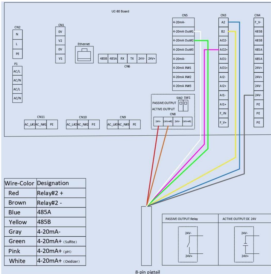
Figure. 5 - Pre-Landed Output Flying Lead Cable Wiring Diagram
