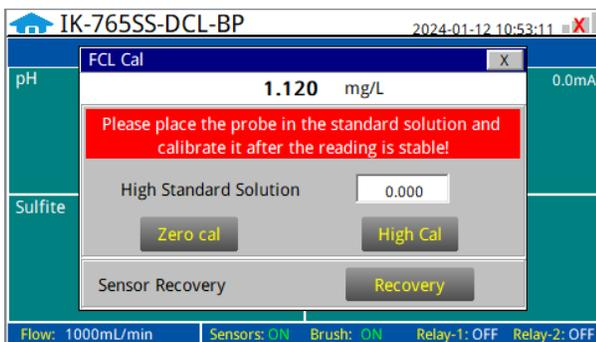
Figure. 43 – Free Chlorine Calibration of ST-765SS-FCL
