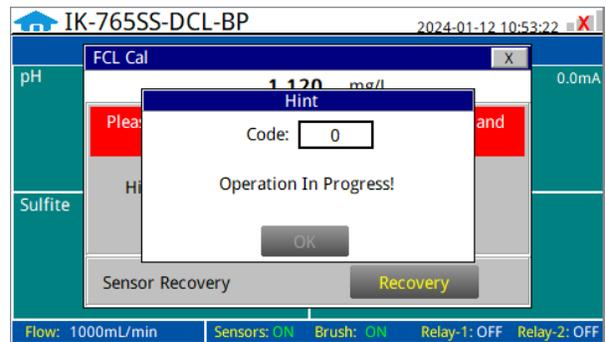
Figure. 44 – In Progress Screen of Free Chlorine Calibration
