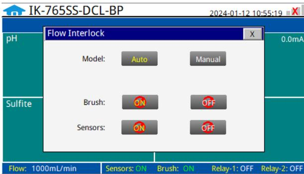
Figure. 18A - Flow Interlock Control - Automatic Mode
