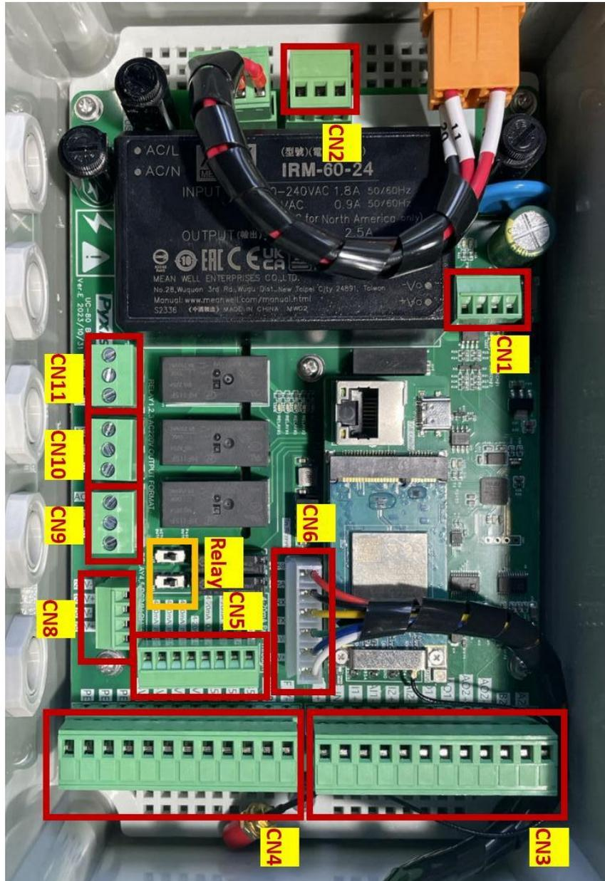
Figure. 3 – Terminal board of the UC-80 Display
